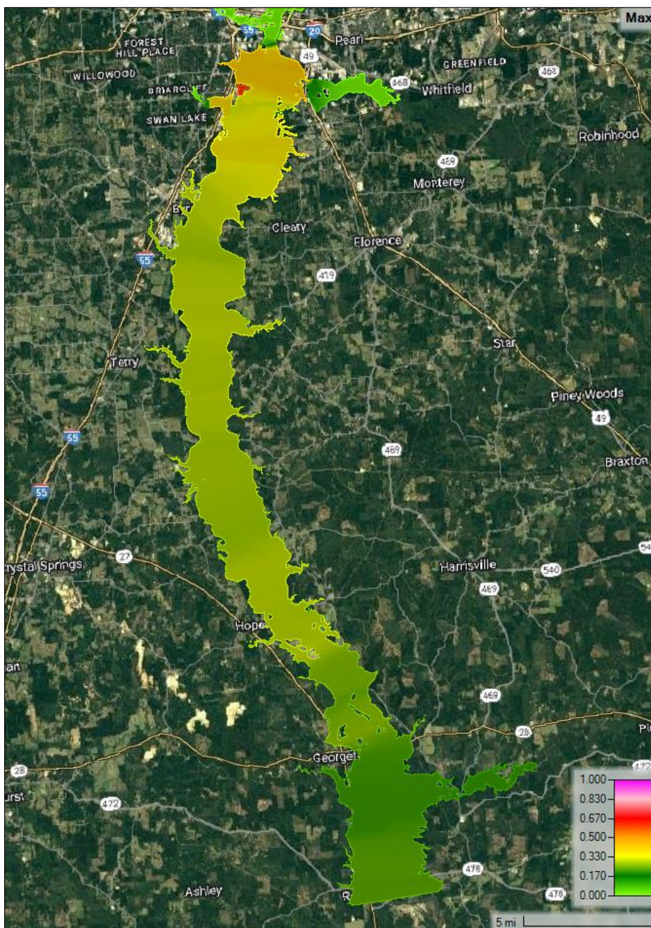
Figure E5-16. 100-year Frequency Absolute Differences (Feet) for With and Without Project. Figure shows the additional height due to Alternative C or CTO construction added to the maximum water surface elevation for the 100-year frequency event. (All areas in green are less than the 0.25 feet, which is considered unlikely to have substantive inducements after further analysis.)
