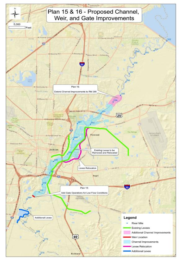
Figure 7-21. Similar to Plan 14, with the addition of gate operations at the weir (Plans 15 and 16) and the
