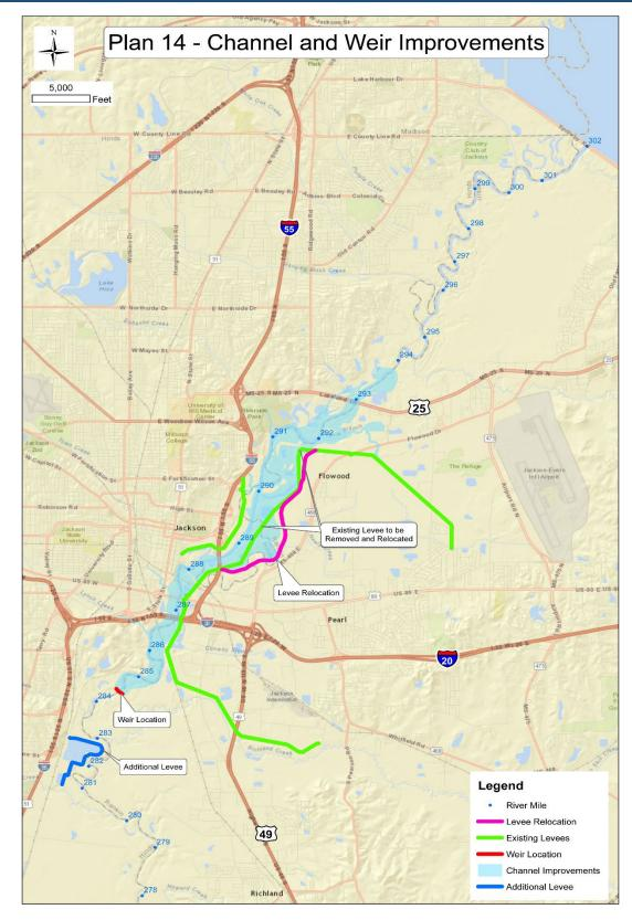
Figure 7-20. Channel improvements from RM 284 to RM 294, with weir relocation and additional levee
