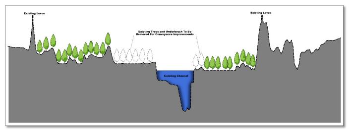
Figure 7-6. Existing trees and underbrush are removed to achieve Conveyance Improvements.
