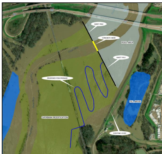
Figure 3-13. Proposed Weir (Black) and Fish Ladder (Blue) Exact Dam Design to be
