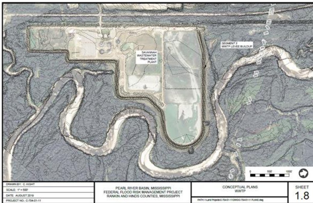
Figure 3-15. Proposed Federalized Levee at Savanna WWTP
