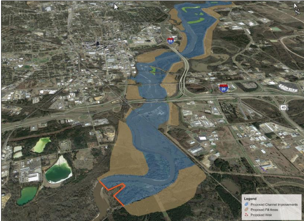
Figure 3-5. Plan View of Proposed Channel Improvements Excavated Material Plan, and Weir with Gate
