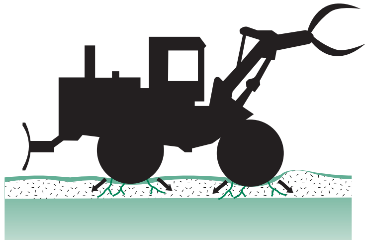
Figure 13. Heavy equipment tires disturb soil during timber harvest. Streambank soils need protection from disturbance, so it is important to keep machinery out of SMZs as much as possible during harvest operations.
